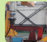
Fatigue life test for connection
