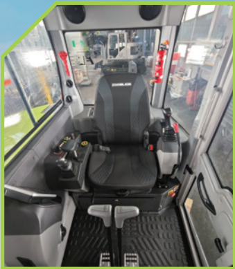
Large space/feature-rich cab + newly designed air duct, large displacement compressor + overall shock absorption in cab + suspension seat
