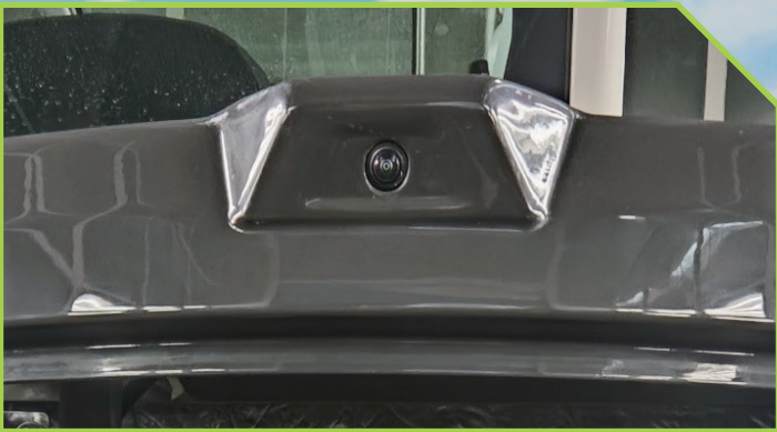
Rearview camera The rearview camera is optional. The rear view is clearly displayed on the monitor, so travel operation is safer.
