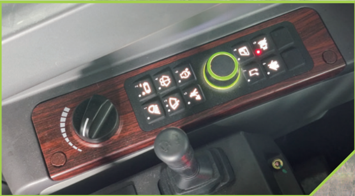
Integrated silicone buttons Silicone buttons and navigation knobs are positioned centralized, so the operation is more comfortable
